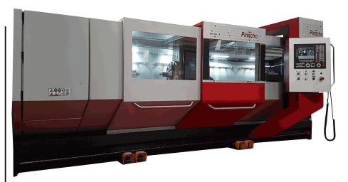
OD-320 X 1800, RPM - 2000, MACHINING **ACCURACY LESS** THAN 0.1 MICRON. **YEAR - 2024** Made in INDIA
